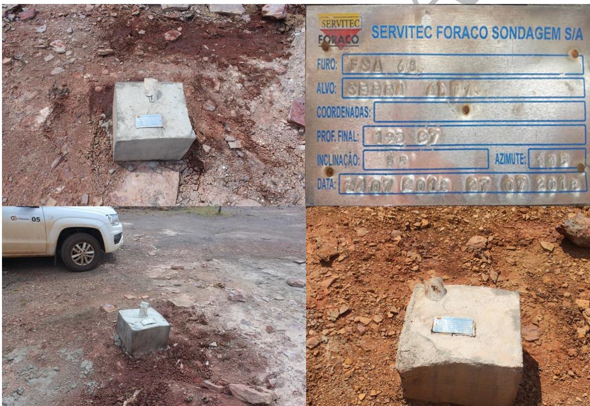
Figure 10.2 Drill Hole Collar Monument
