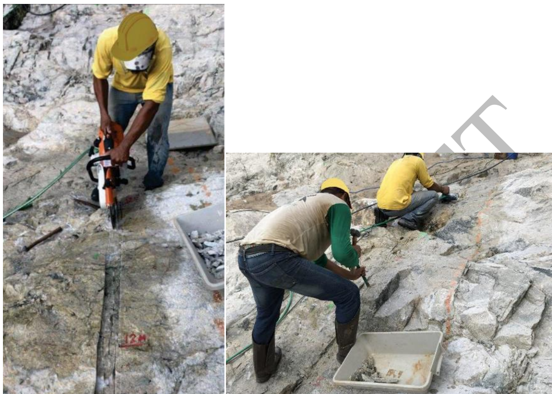
Figure 9.14 PNP Channel Samples Collected in Hard Rock Using Electric Saw with Diamond Blade
