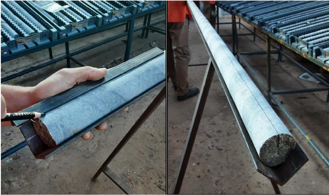
Figure 10.9 Drill Core Orientation Process
