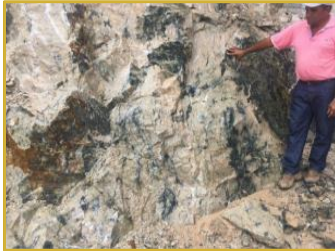
Sheared Granitic ore with sulphide rich quartz, chlorite veining.
