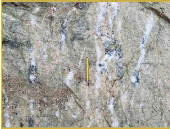
Sheared Granitic ore with sulphide rich quartz, chlorite veining.
