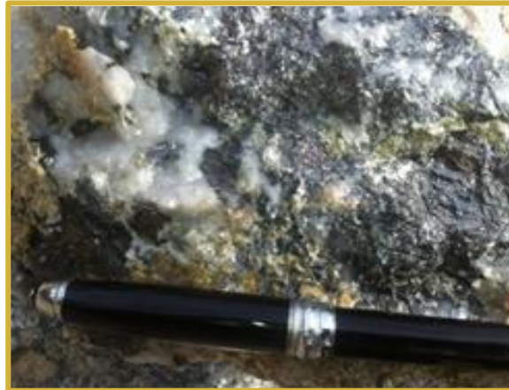
Sheared Granitic ore with sulphide rich quartz, chlorite veining.
